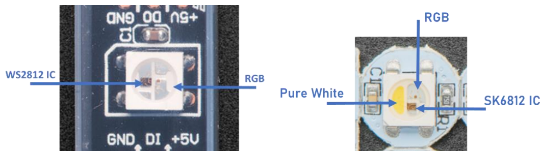
Figure 3-13: WS2812 LED vs SK6812 LED light Set Up
