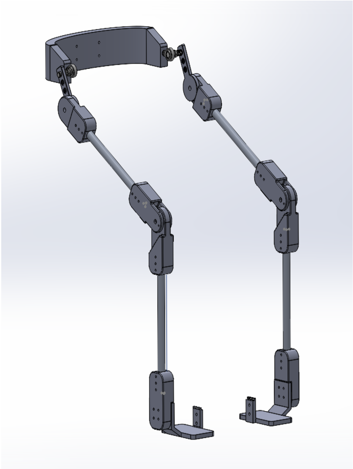
Fig 2: Rough model of our lower body exoskeleton design. With fully functional and motorized hip and knee joints, and a battery pack with User Interface located on the back panel.
