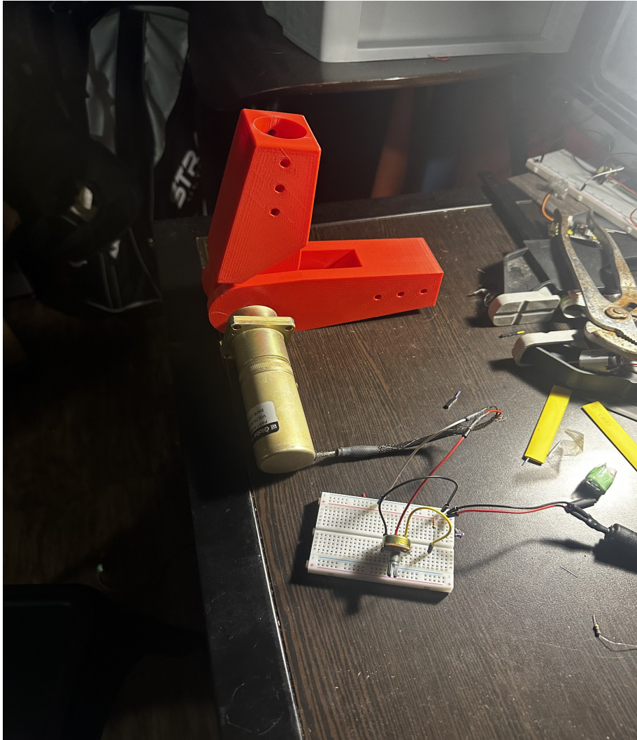
Figure 3.9.2 DC Brushed Motor Test with 3D Printed Joint
