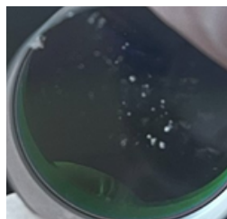
Figure 9.1 Dichroic Mirror Test Damage
