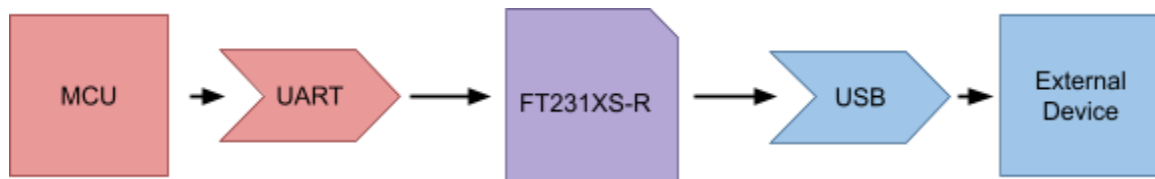
Figure 6.5 Data output Subsystem Block Diagram
