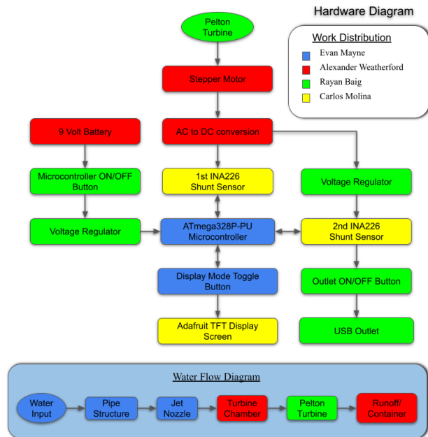
Fig. 2. This hardware diagram shows the connections between the electrical components electrical and the water based mechanical components.
