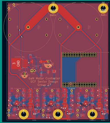
Motor Controller Power PCB
