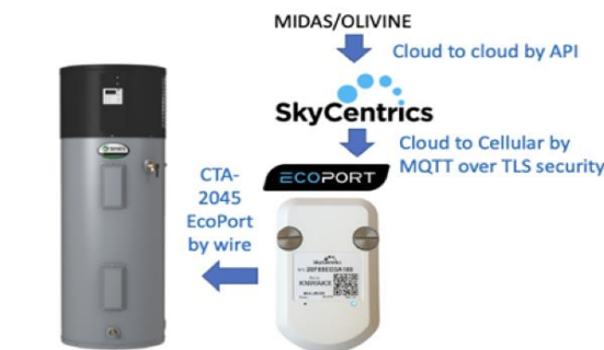
Figure 1: CTA-2045 device diagram
