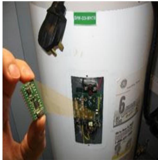
Figure 2: Grid Friendly Appliance chip retrofitted to Water Heater
