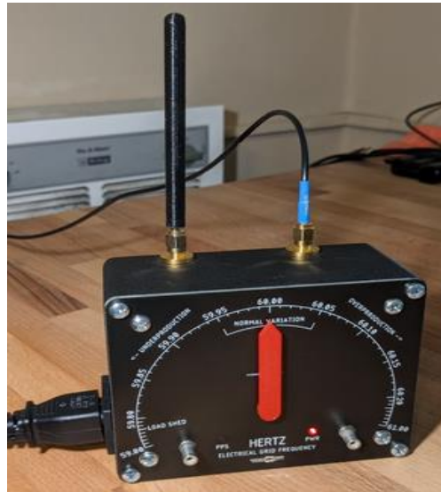
Figure 3: Analog frequency detector
