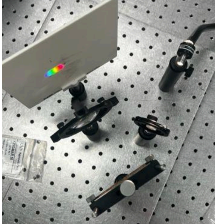
Figure 8.7: Basic Spectrometer Layout used for Prototyping
