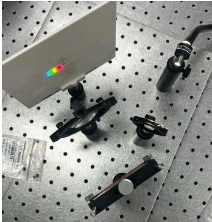
Figure 8.7: Basic Spectrometer Layout used for Prototyping
