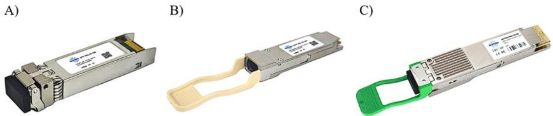
Figure 3.18 Examples of different form-factor modules. A) SFP+ module. B) QSFP+ module. C) QSFP-DD module. Fig. created by Authors of images collected from Ref. [149].
