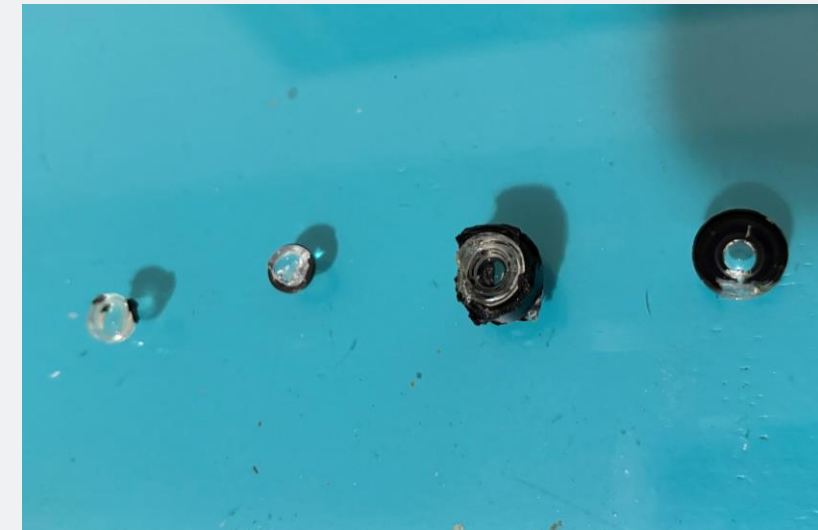
Lenses from an off-the-shelf surveillance camera
