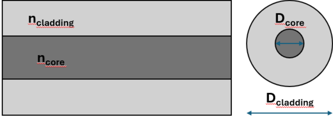
Figure 3.19. Simplistic optical fiber schematic showcasing the refractive index difference between core and cladding and between core and cladding diameters. Figure by Authors.
