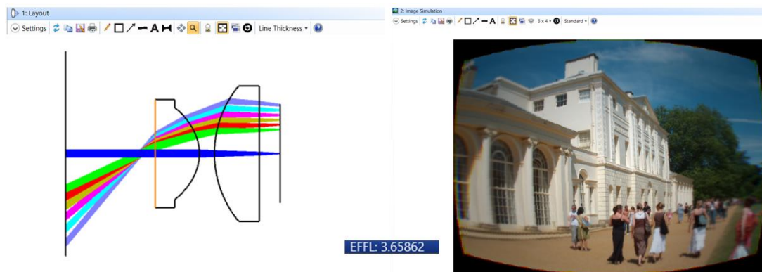
Figure 9.6. Final lens design for iSPY (Zemax output).
