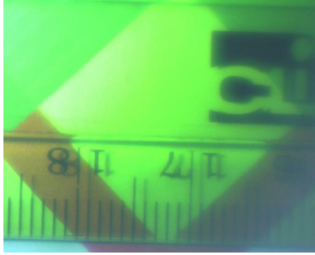
Figure 8.2. Frame taken by the laptop connected to the CMOS sensor. A ruler was imaged onto the sensor, we can only see the bottom part of it.
