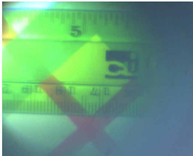
Figure 8.4. Frame taken by the laptop connected to the CMOS sensor. A ruler was imaged onto the sensor, and we can see the top and bottom of it.
