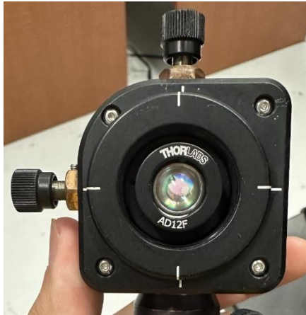
Figure 6.10. Kinematic mount with a collimator lens ready to use in a free-space link.
