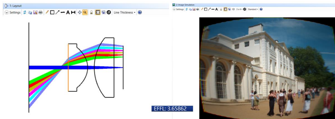
Figure 9.6. Final lens design for iSPY (Zemax output).
