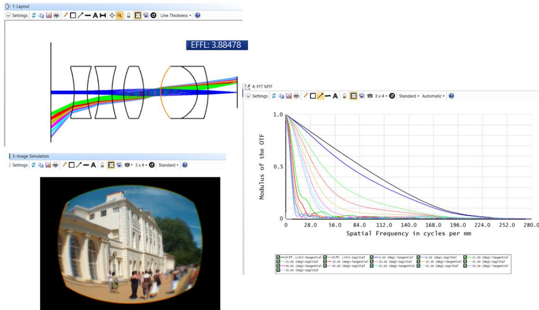
Figure 9.5. Attempt on inverted telephoto lens system with an achromatic lens (Zemax output).
