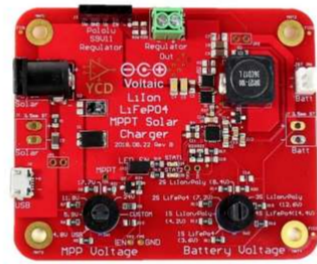
Figure 3.4.4b: Voltaic System Solar Charger
