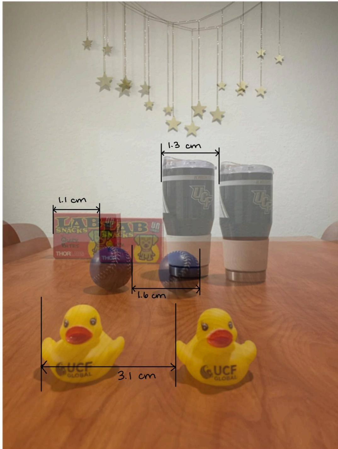
Figure 9.1.3c: Overlay of the left and right camera images, being used to measure the disparity between objects in the image
