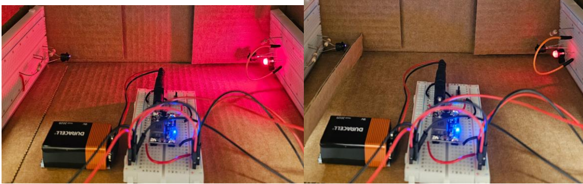
Figure (9.2) - Break-beam sensor test, system-on(left). System with a cardboard piece placed in between of IR LED and photodetector showing the much dimmer red LED.
