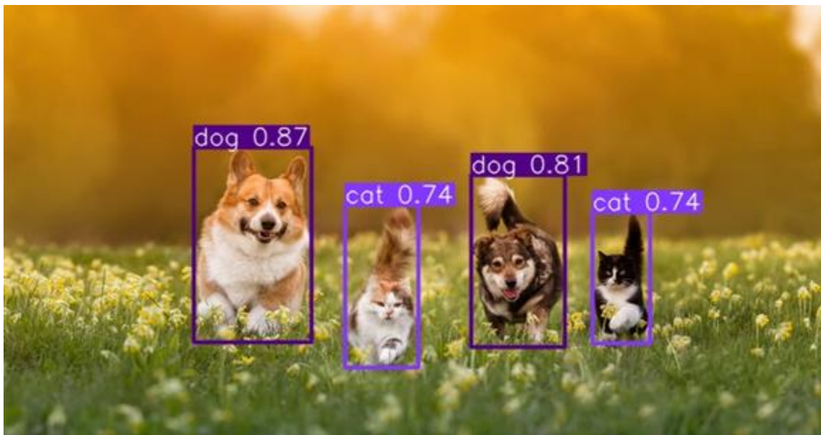
Figure (9.1) - Prototype testing image from Adobe Stock of two cats and two dogs running through a flower field. This image has confidence level bounding boxes from the medium model.
