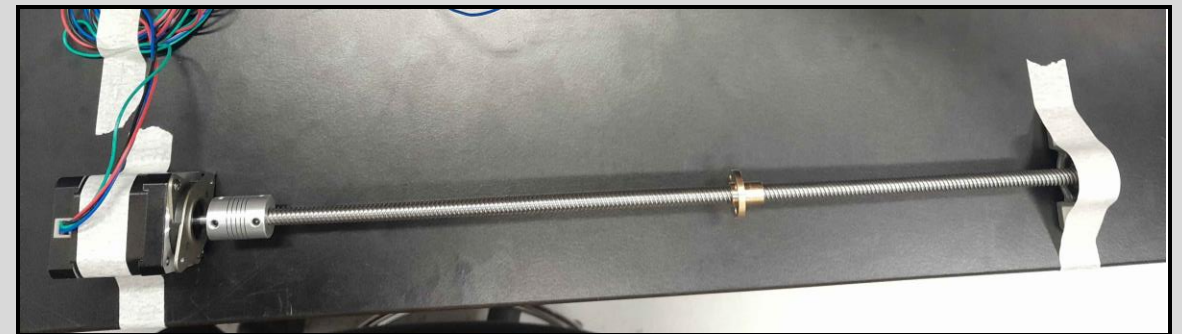
Fig 3. 400-mm lead screw linear actuator to be used in P.A.W.S. rail system
