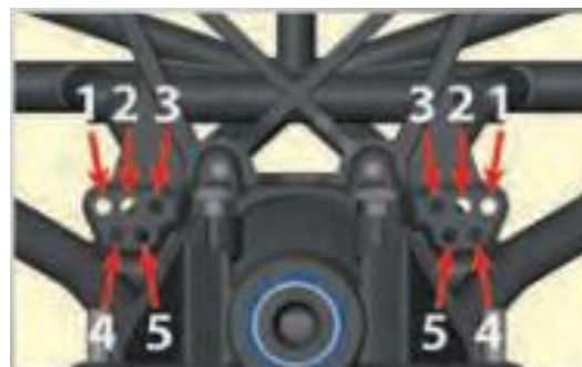
Figure 6.1.3.2: Rear suspension, roll center adjustment point. Source: [125]
