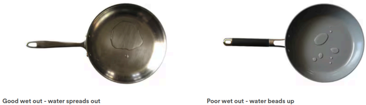
Figure 3.1.19.2: Good vs. Poor Wet Out [73]
