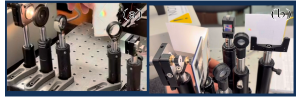
Fig. 9. Optical prototype evolution for the monochromator subsystem. (a) First prototype. (b) Second prototype
