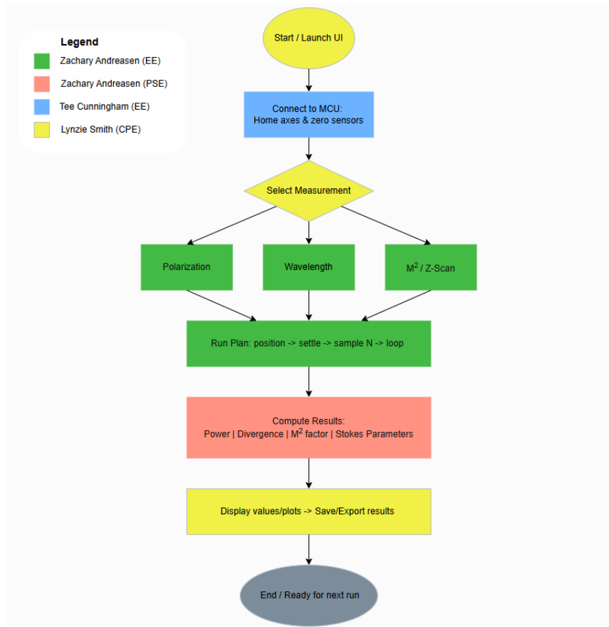
Figure 4: Laser Beam Characterizer Software Block Diagram
