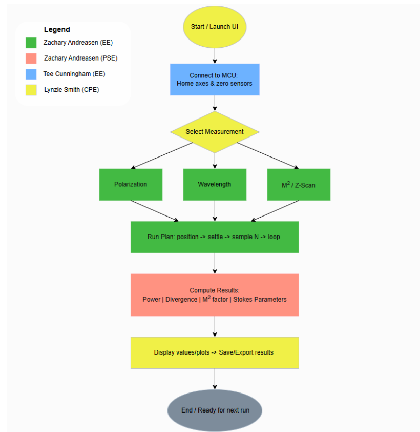
Figure 4: Laser Beam Characterizer Software Block Diagram
