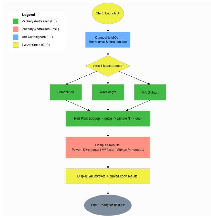
Figure 4: Laser Beam Characterizer Software Block Diagram
