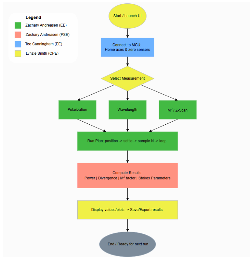
Figure 4: Laser Beam Characterizer Software Block Diagram
