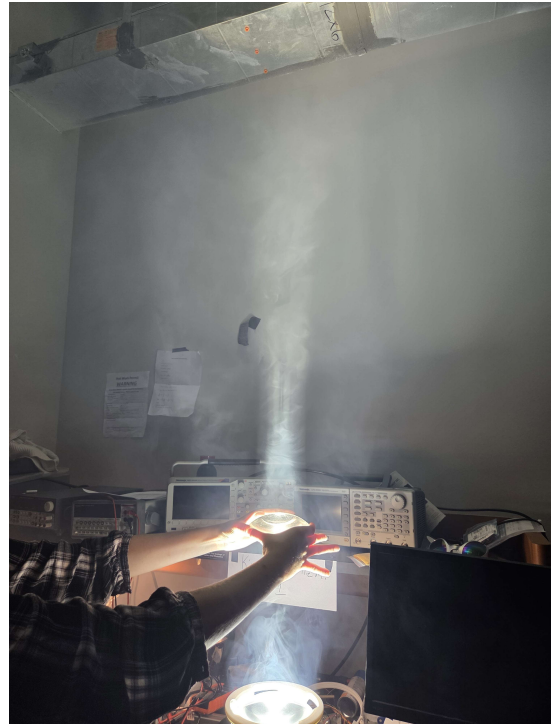
(d) Semi-collimated beam created via a beam compressor configuration
