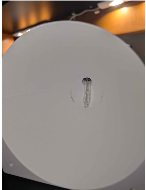
(b) HID bulb is mounted at an angle in the reflector.
