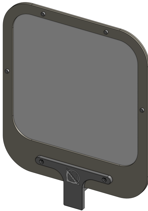
Fig. 32: Image assembly model, features a sheet of paper sandwiched between laser cut wooden panels. Working image area is 200 x 200mm.
