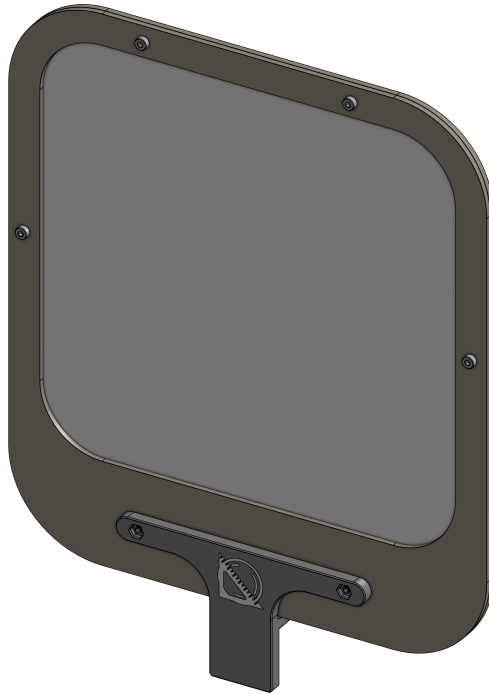
Fig. 37: Image assembly model, features a sheet of paper sandwiched between laser cut wooden panels. Working image area is 200 x 200mm.
