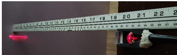
Figure 7: Laser cursor optics mount (alignment testing)
