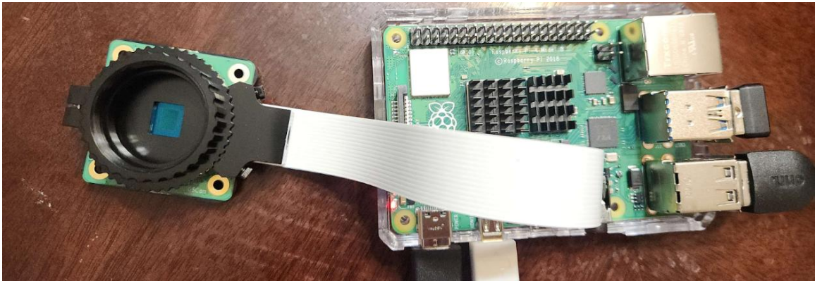
Figure 51: Global Shutter CMOS sensor module attached to SBC
