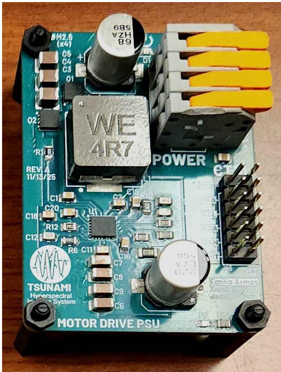
Figure 38: Picture of finalized motor driver PSU circuit board
