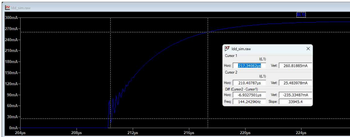
Figure 18: Laser diode current rise time measurement, hitting 7μs!
