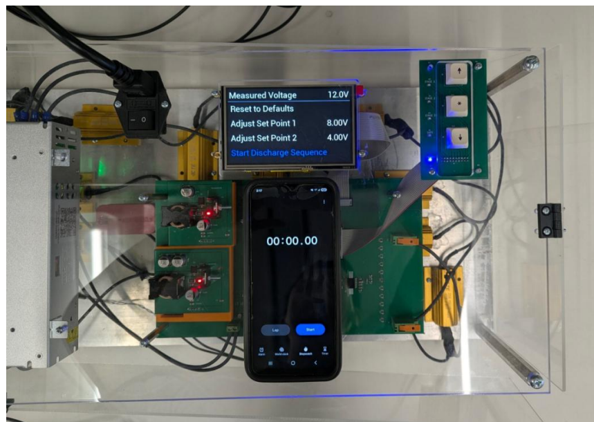
Figure 54: Discharge Time Test Setup
