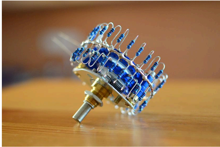
Figure 3.14: “DIY stepped attenuator of the shunt type made with 0.5 watt metal-film resistors” by Dimitar Sumerski from audio-at-home.com [104]
