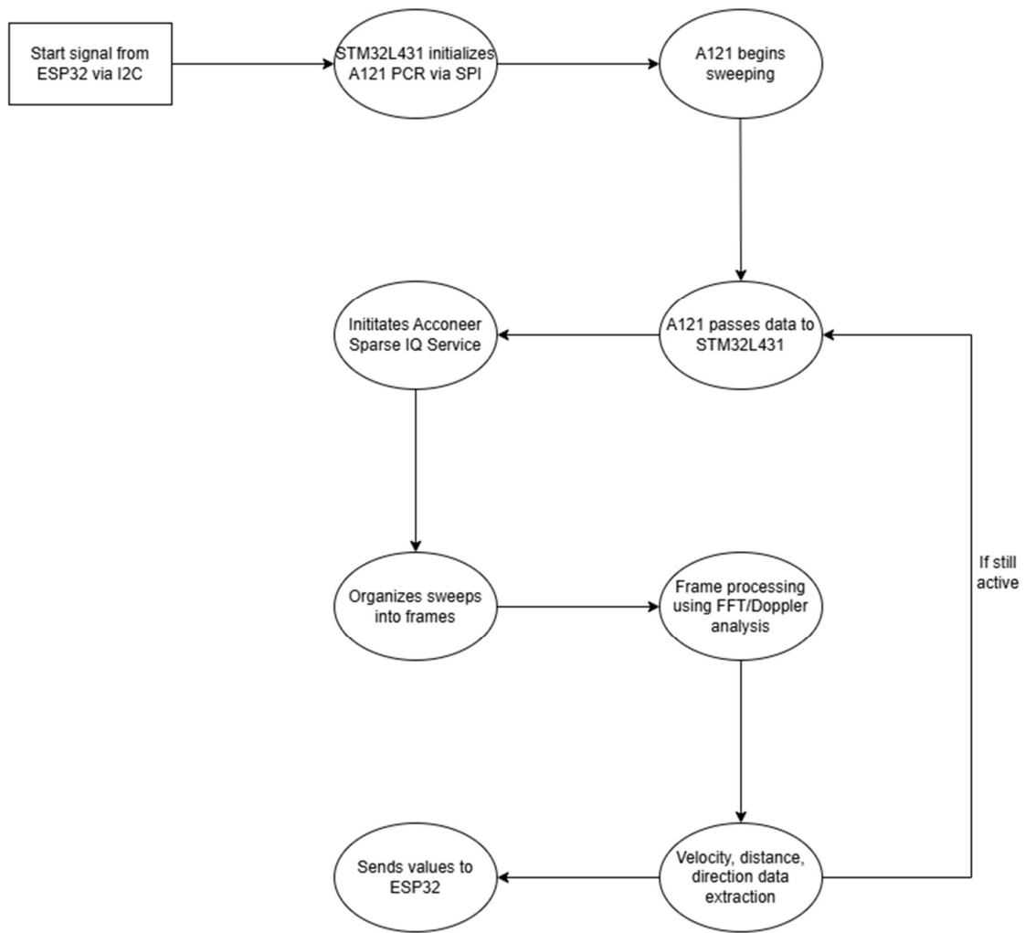
Figure 28 – XM125 Radar Software Flowchart.
