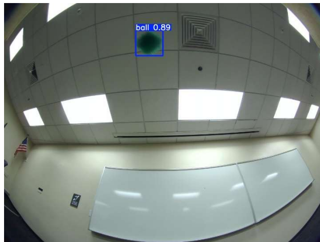
Fig.3. One of the playground balls was detected on the wide-angle camera mid-air. The model had a confidence of 89%, which is reasonably high. The remaining images captured during the rest of the throw showed similar results.
