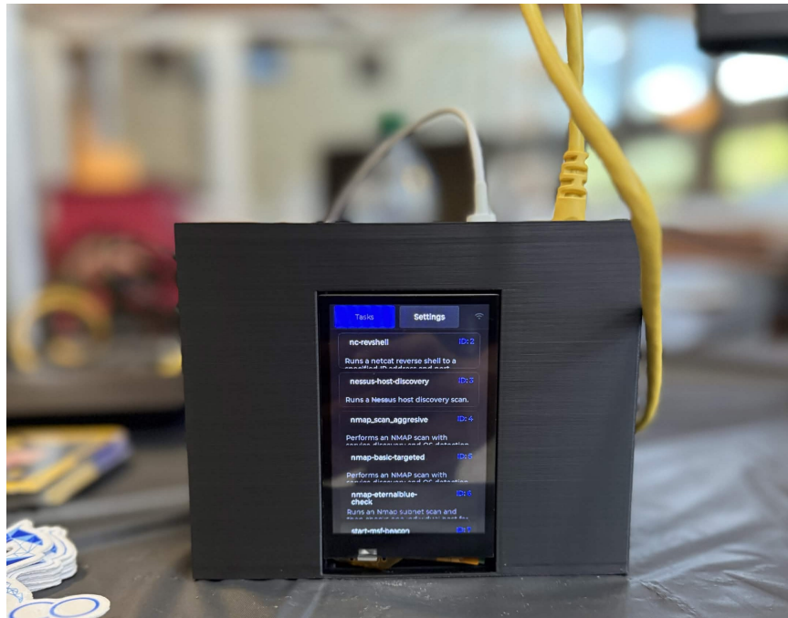
Figure 22: Front view of the PWNBoxer prototype showing the embedded display interface used for user interaction, task execution, and real-time system feedback.
