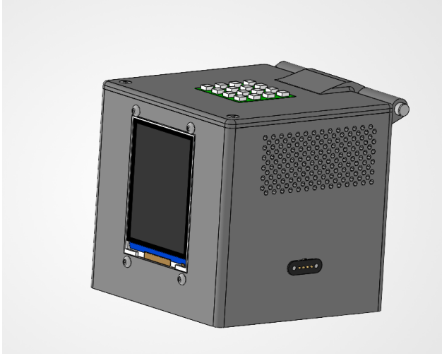
Fig. 4. External SolidWorks model showing the TFT display, LED matrix, and pogo-pin interfaces.
