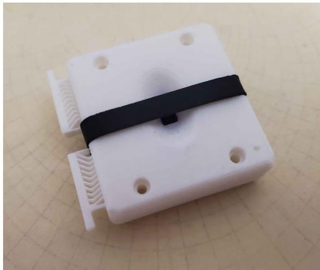
Fig. 3. Prototype model of the PPG module's case.
