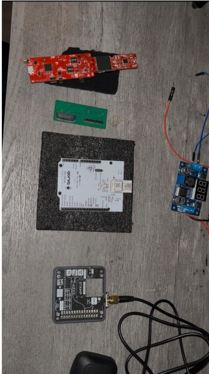
Figure 37: Components acquired aside from those listed above: Radar module, UWB sensor, INS.
