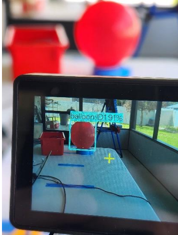
Figure 4. Showing what the HuskeyLens sees and even with two red object in its frame, it only puts a bounding box around the Ballon.
