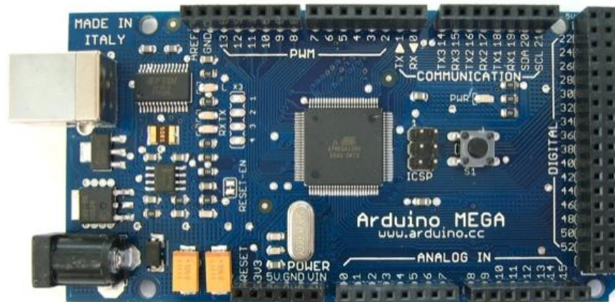
2.2.3 Figure 2: Arduino Mega microcontroller used with permission from Arduino
