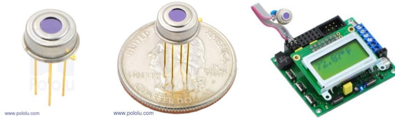
Figure 4.2-3 MLX90614 reprinted with permission by Pololu.com
