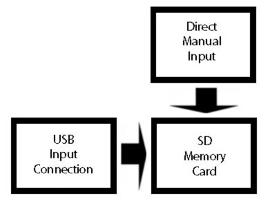
The input unit will be our path way to interaction with the LED cube. Here animations can be loaded into a dedicated SD memory card either through a provided USB connection or by directly installing the animations on the SD card. The SD card will hold all of the desired animation that will be fetched by the control unit for processing and future display.
