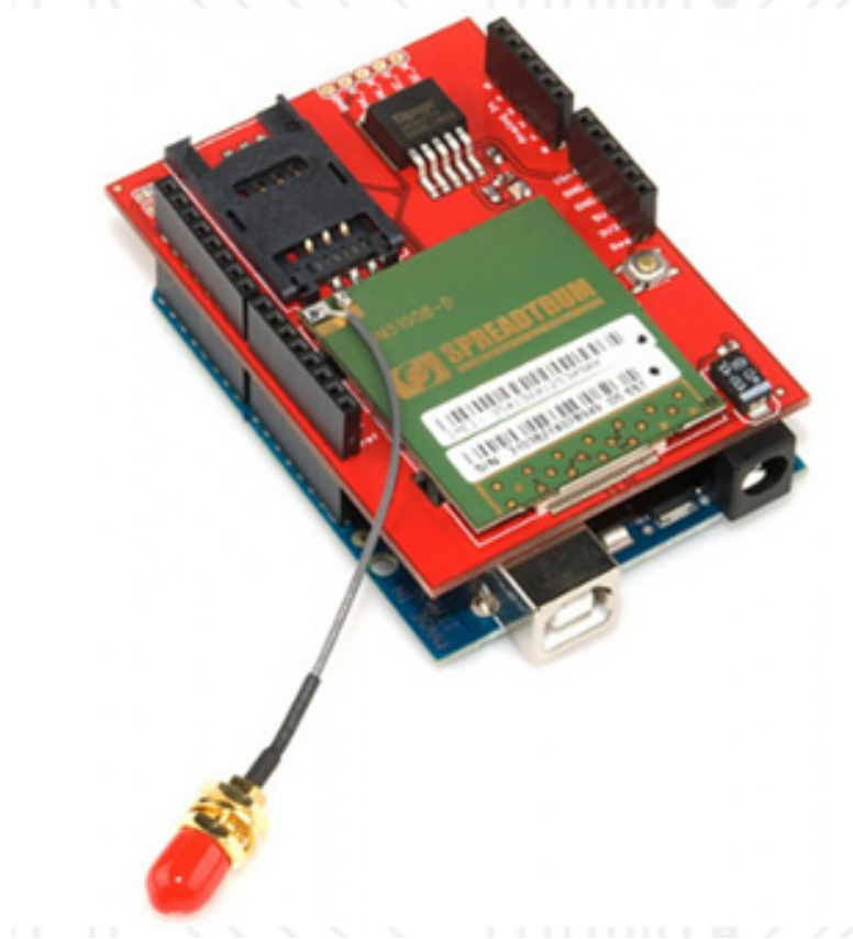
Figure 32: the Cellular Shield (SM5100B) with Arduino Printed with permission from an open source Sparkfun.com
