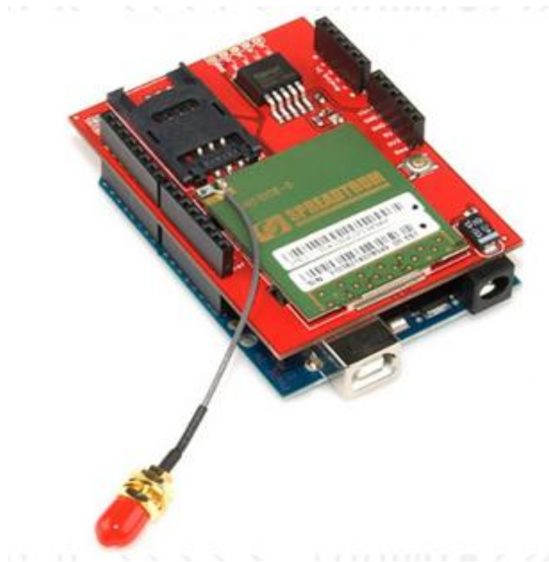
Figure 37: the Cellular Shield (SM5100B) with Arduino
