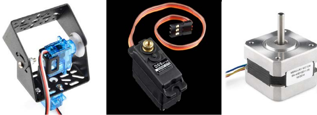
Figure 3-5 – Pan and Tilt ( left ), Servo ( center ), Stepper ( right ) (Reprinted with permission from SparkFun Electronics)
