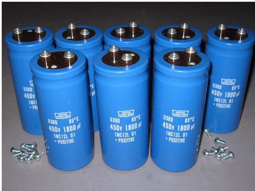
Figure 4-19 – Capacitors Chosen for the Capacitor Bank
