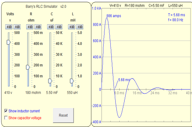
Fig. 2 RLC Simulator showing current pulse. (Reprinted with permission from Barry Hansen).
