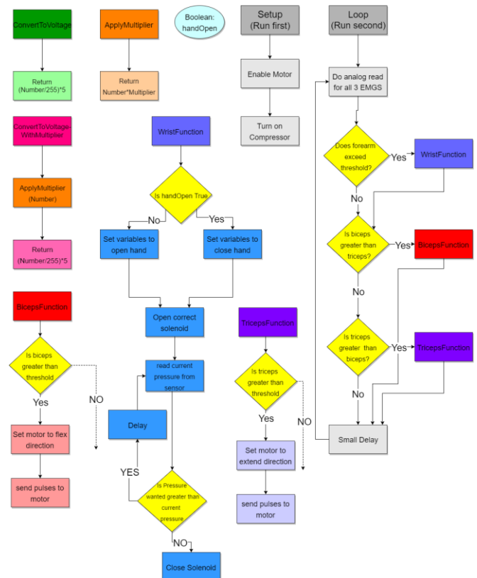
Software Low Level Design 1. This is a flow diagram of how the system will be coded.
