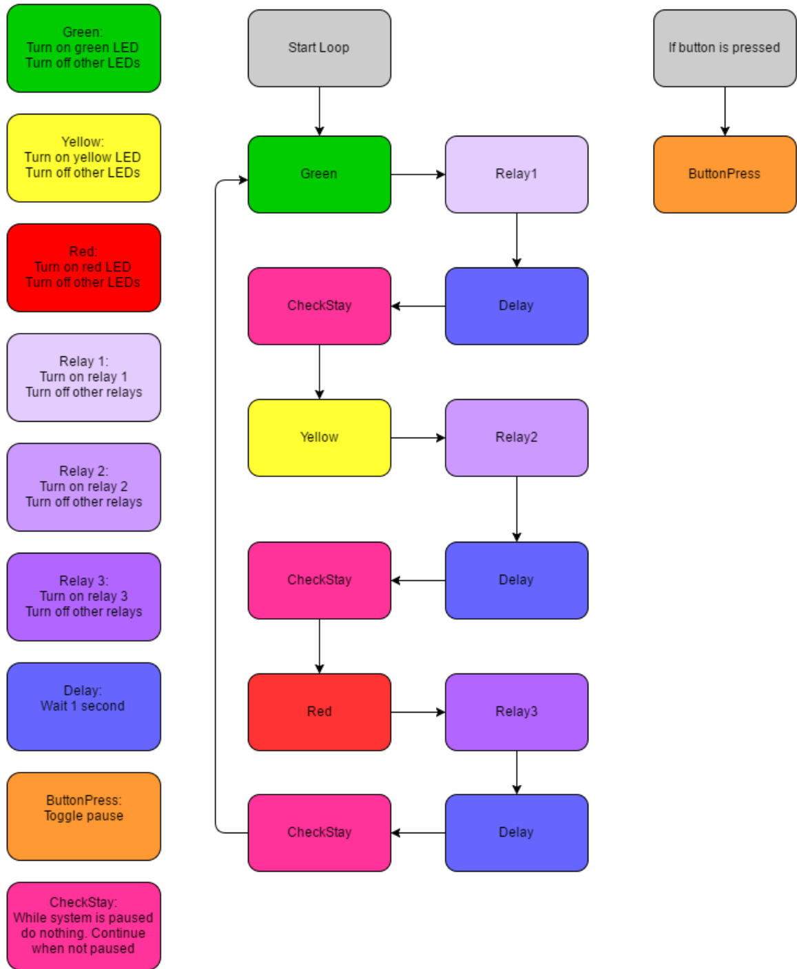
Code Research 1. This is a diagram of the code written to test the basic functions of the Arduino. These functions include input, output, and interrupts.
