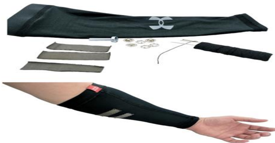
Electrodes 1: Conductive sleeve concept put together by the mechanical team
