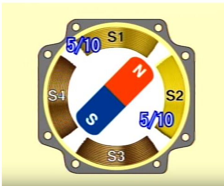
Stepper Motor 1: Maximum Current Rotor Position Image from youtube.com
