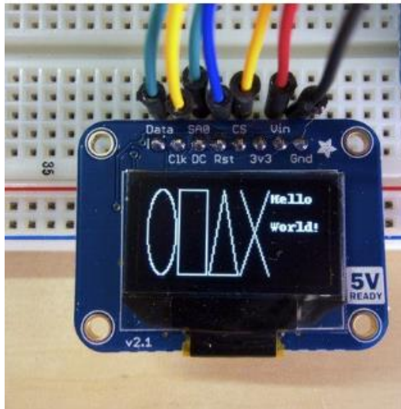
Figure 75: OLED Display demonstration executing shapes.py
