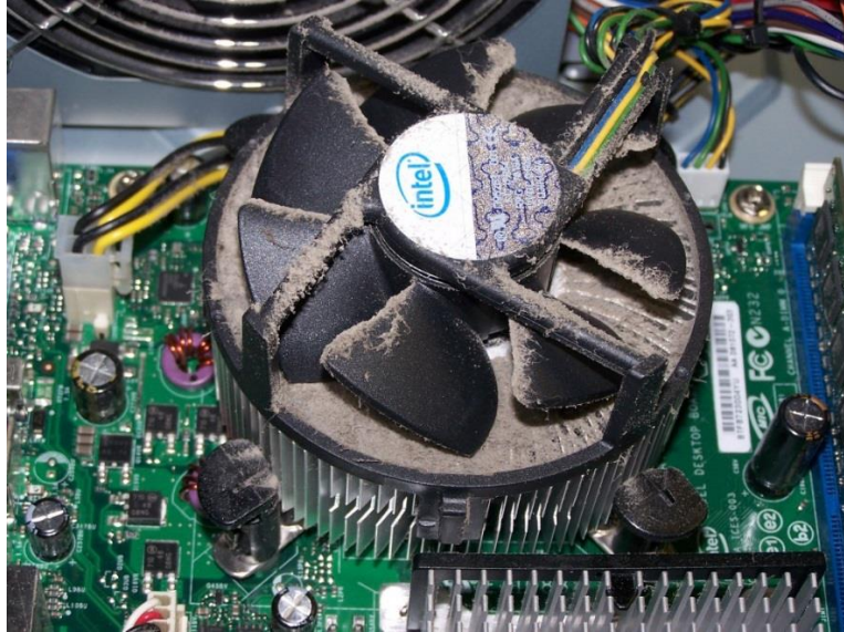
Figure 2. Cooling fan system with no maintenance [39] Courtesy of dirtycomputer.com
